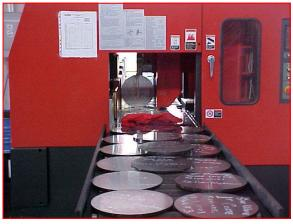
With self-feeding action, the band actually grows in width (see magnified back edge view of the SineWave<sup>®</sup> blade above), forcing each tooth to penetrate the work more efficiently.
