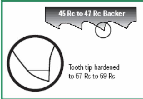
**DieBand Plus** incorporates 8% cobalt high speed wire on a high tensile strength spring backer to provide longer blade life. **DieBand Plus** can be welded with a standard blade welder or a high speed welder.
